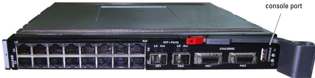
Figure 2. Connecting to the Console Port
